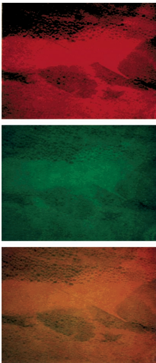
Figure 4. Fluorescence microscope image of an \alpha -lactalbumin/ \beta -casein mixed protein film at the air–water interface: (A, top) image taken with a red filter; (B, middle) image taken with a green filter; (C, bottom) image taken with a mutual filter. The surface concentrations of \alpha -lactalbumin and \beta -casein in the mixed film were about 0.12 and 1.1 \text{mg m}^{-2} , respectively, corresponding to initial bulk concentrations of 0.15 and 1.5 \mu\text{g/mL} , respectively. The color schemes and scale are as in Figure 2.
